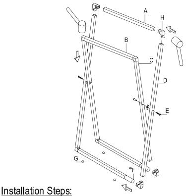
Step1. Straight tubes by length, you should have 2 of each length, insert a counterweight rod (part F) into a tube A (15-1/8") and one into tube B (13-1/2"), make sure each tube has two small holes on one side.
